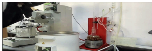
Figure 2: Clevenger hydrodistillation apparatus used for the extraction of essential oils from Rosmarinus officinalis L.
